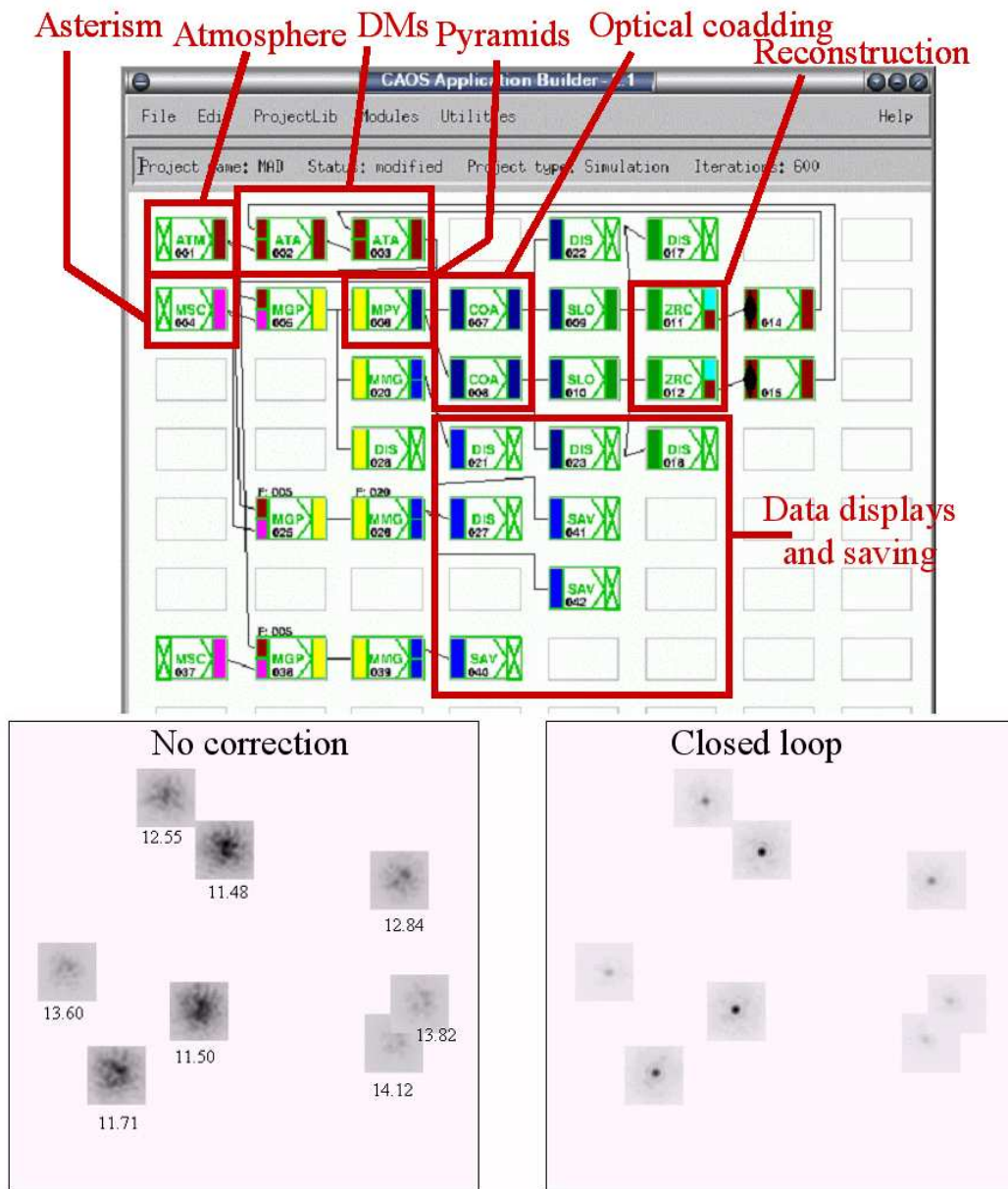
Figure 4. Top: the CAOS Application Builder showing a typical simulation design using the modules of the Software Package MAOS for simulating the ESO MCAO demonstrator MAD, in LO mode. Bottom: the result of the simulation in terms of PSF shape in the sensing field (sensing magnitudes are also marked).
