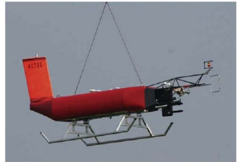
Fig. 1. ACTOS comprises instrumentation for comprehensive measurements of thermodynamic, microphysical, and turbulent variables in clouds, at high spatial resolution. The ACTOS measurement payload is attached to the helicopter by means of a 140 m long tether cable. The true airspeed of the helicopter is about 15 m/s, sufficient to enable stable flight conditions of ACTOS out of the helicopter's downwash.
